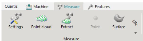
The point clouds are the basis for the extraction of geometric elements and thus an important elementary function for optical measurement. You will already be able to extract geometry elements from the point clouds in WM | Quartis R2021-1.
